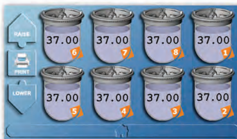
Individual vessel temperature readings with DTPs
