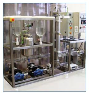
provided by Solvionic. The project will look to develop a highly energy-efficient microwave flow reactor and demonstrate its application using ionic liquid-based processes.
