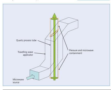
Figure 1 - Microwave cavity
